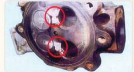
Cylinder Head of MW Engine, crack in combustion chamber repaired by Metal Stitching
